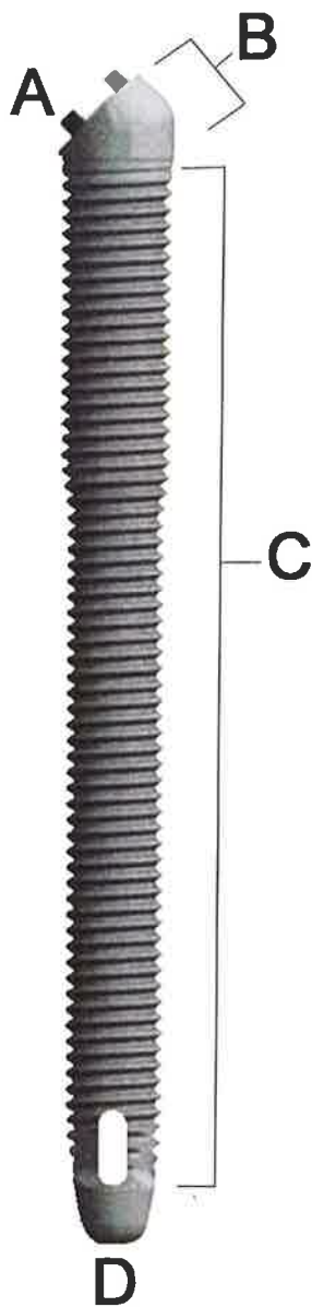
Figure 7: The Brånemark System Zygoma Implant: (a) regular platform external hex connection, (b) prosthetic access is at a 45° angulation from the long axis of the implant, (c) the implant body consists of two diameters [4.6 mm at the coronal or maxillary end; 3.9 mm at the apical or zygomatic end], (d) the apex is a rounded tip to prevent sharp edges when the implant penetrates the lateral wall of the zygoma.
